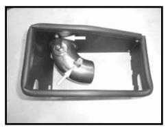
Step 6 Install L bracket to tube and heat shield. Wait to tighten until a later step. Also install the supplied grommet into the intake tube then install IAT sensor into the grommet.
