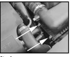
Step 3 Unclip the two hold down clips on the air box lid and remove it for the vehicle.
