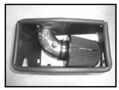
Step 7 Install the supplied air filter and clamp and tighten the clamp that secures the air filter.
