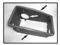
Step 5 Install the provided edge trim onto the heat shield as shown in picture.
